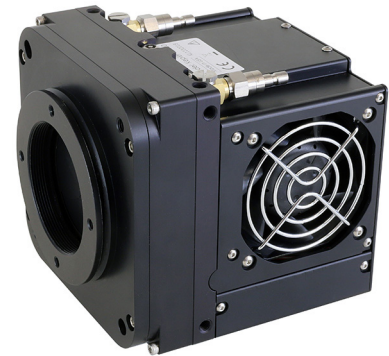
KL400 with Optional 45mm Shutter
