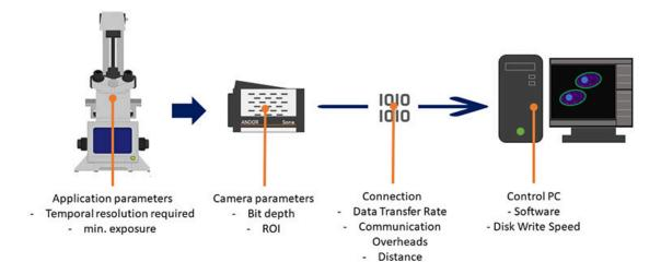
What are the different camera interfaces that link to the control PC and why are there so many different types? Each connection has the same objectives:
