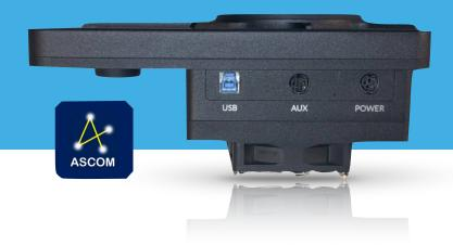
The SBIG STC-428 scientific CMOS Active Pixel Sensor cameras represent a major improvement over CCD technology. Compared with previous CCD models such as the STF-8300M, the STC-428-P features higher sensitivity (78% QE versus 56%), significantly lower read noise (2.5 e- versus 9.3 e-), and 20X faster readout.
